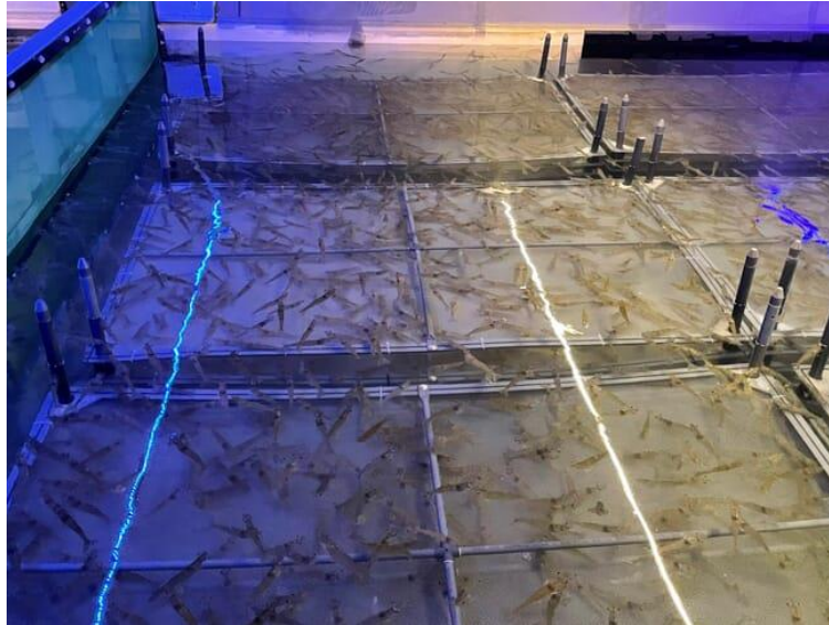
Wecker uses a u-turn raceway system in his RAS design
